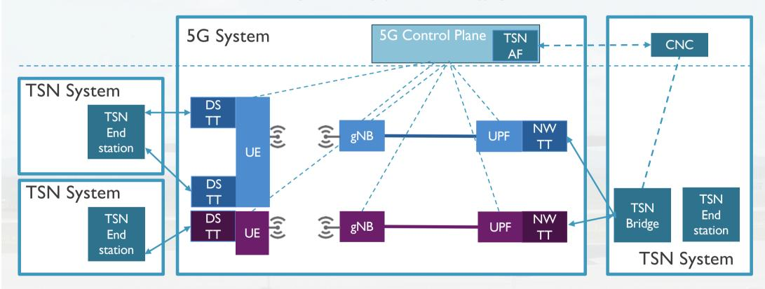
CNC - Central Network Controller | UPF - User Plane Function | AF - Application Function | DSTT - Device Side TSN Translator | NWTT - Network Side TSN Translator
